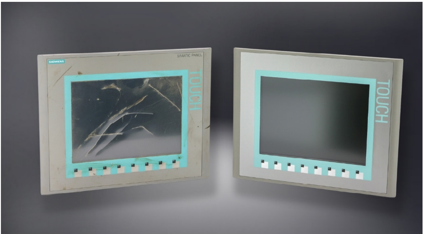
Damaged HMI (left) and revised HMI (right)
