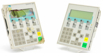
Damaged and revised membrane control unit
