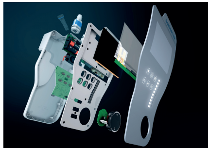
Construction of an HMI PCAP input system
