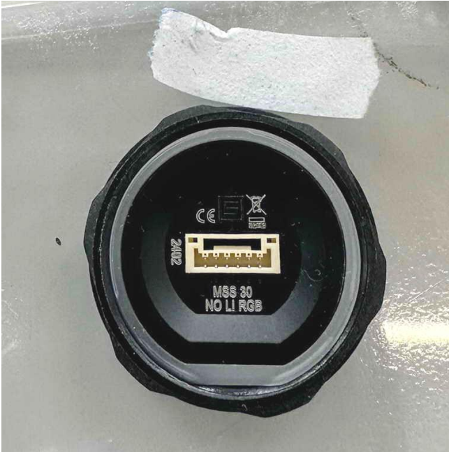
Fig. 74 Sample 7 dry test after IPX9K pos. 1.
