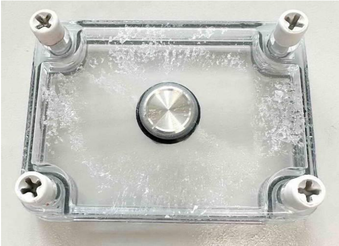
Fig. 34 Sample 3 after IP6KX, view 2.
