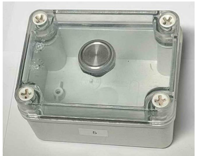
Fig. 51 Sample 5 after IP6KX, view 1.
