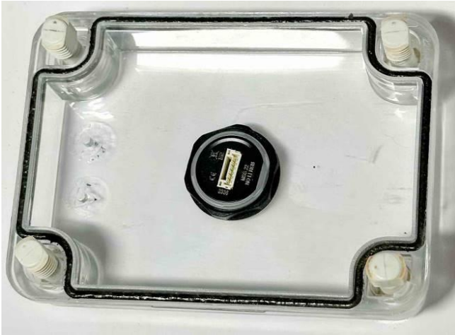
Fig. 52 Sample 5 after IP6KX, view 2.
