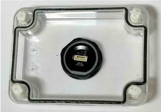
Fig. 70 Sample 7 after IP6KX, view 2.
