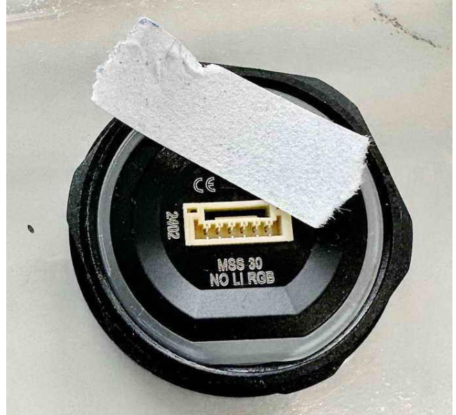
Fig. 75 Sample 7 dry test after IPX9K pos. 2.
