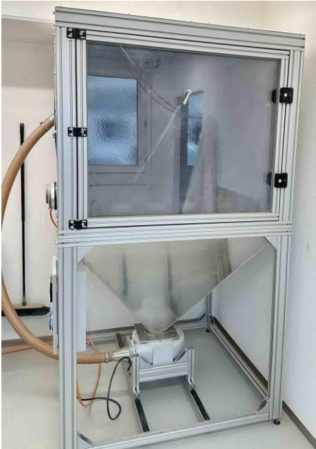
Fig. 1 Arrangement IP6KX, test chamber with DUT.
