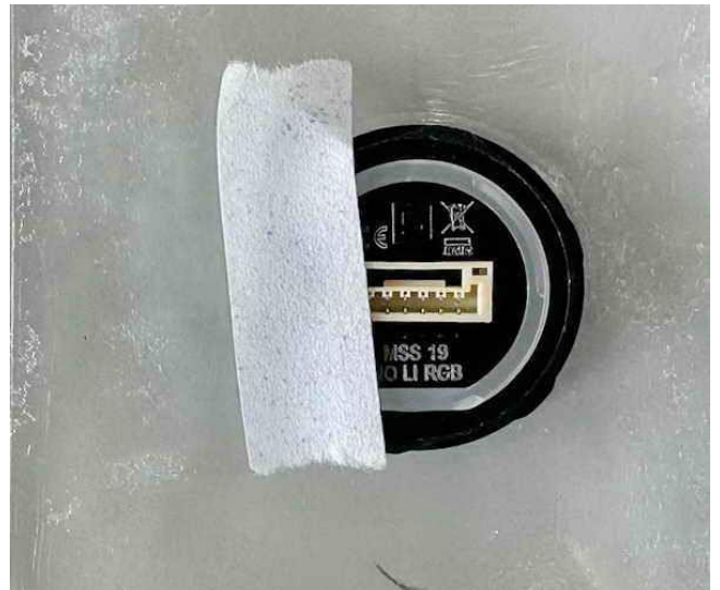
Fig. 48 Sample 4 dry test after IPX9K pos. 2.
