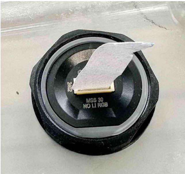
Fig. 76 Sample 7 dry test after IPX9K pos. 3.
