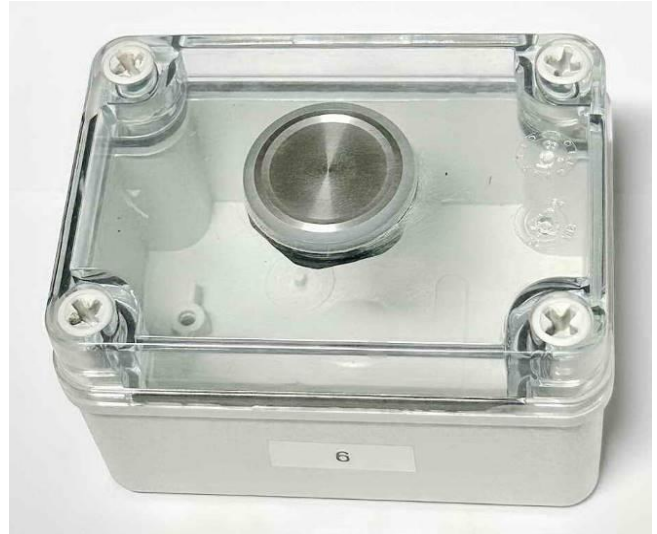
Fig. 60 Sample 6 after IP6KX, view 1.
