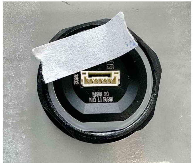
Fig. 66 Sample 6 dry test after IPX9K pos. 2.
