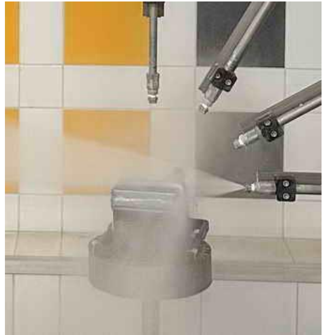
Fig. 13 DUT during spraying 0°, IPX9K.
