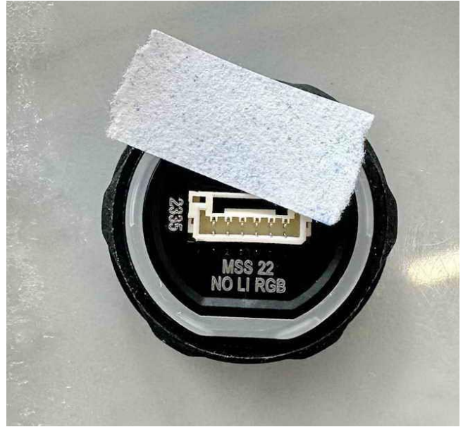
Fig. 57 Sample 5 dry test after IPX9K pos. 2.
