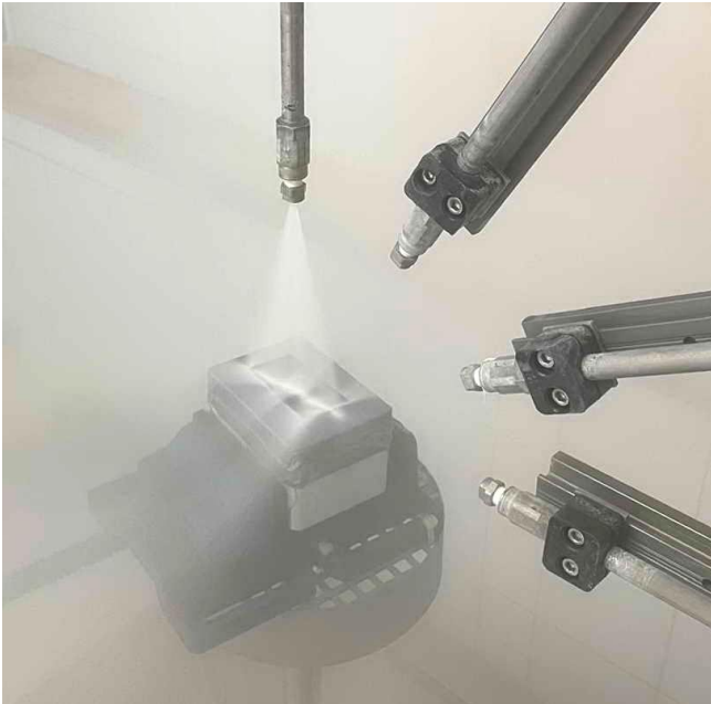
Fig. 10 DUT during spraying 90°, IPX9K.
