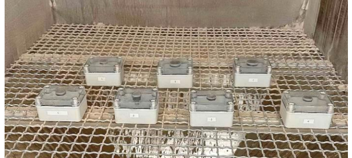
Fig. 9 DUT at the end of test application IP6KX, excess dust removed.
