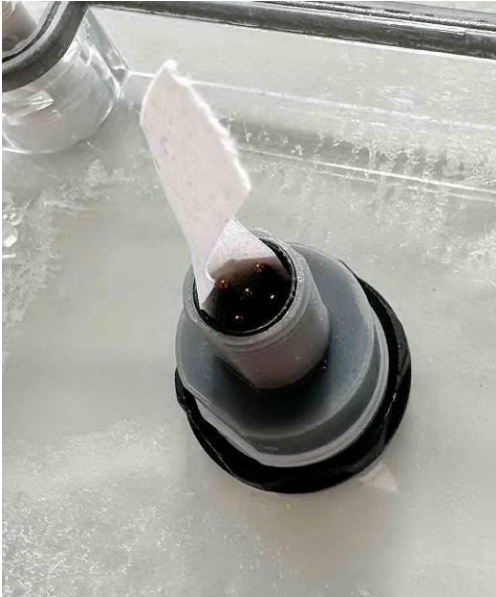
Fig. 31 Sample 2 dry test after IPX9K pos. 3.
