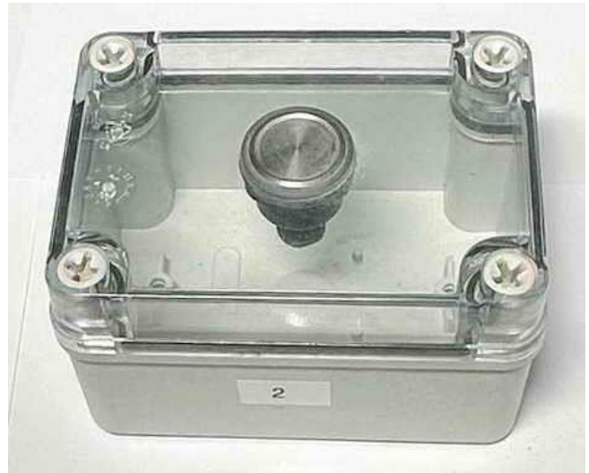
Fig. 24 Sample 2 after IP6KX, view 1.
