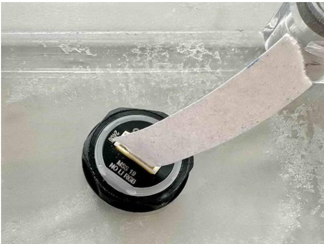
Fig. 40 Sample 3 dry test after IPX9K pos. 3.
