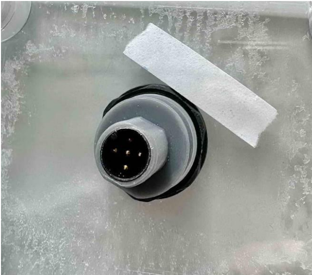
Fig. 29 Sample 2 dry test after IPX9K pos. 1.
