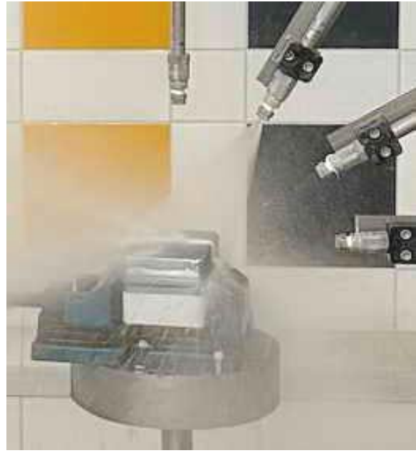
Fig. 11 DUT during spraying 60°, IPX9K.
