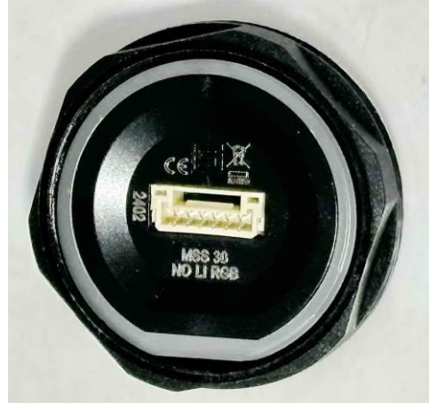
Fig. 62 Sample 6 after IP6KX, view 2_1 detail.
