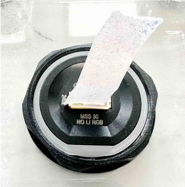
Fig. 67 Sample 4 dry test after IPX9K pos. 3.
