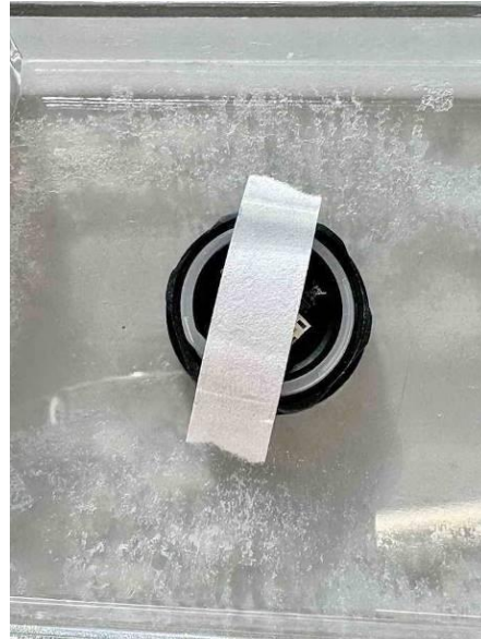
Fig. 21 Sample 1 dry test after IPX9K pos. 2.
