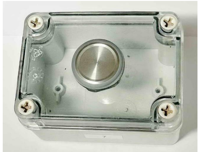
Fig. 69 Sample 7 after IP6KX, view 1.
