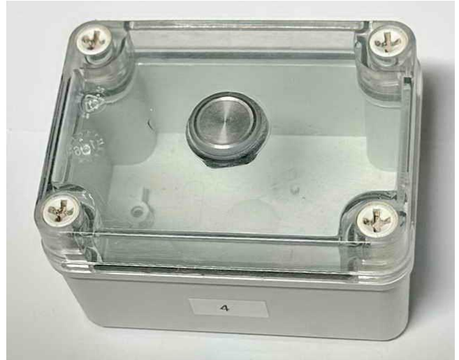
Fig. 42 Sample 4 after IP6KX, view 1.
