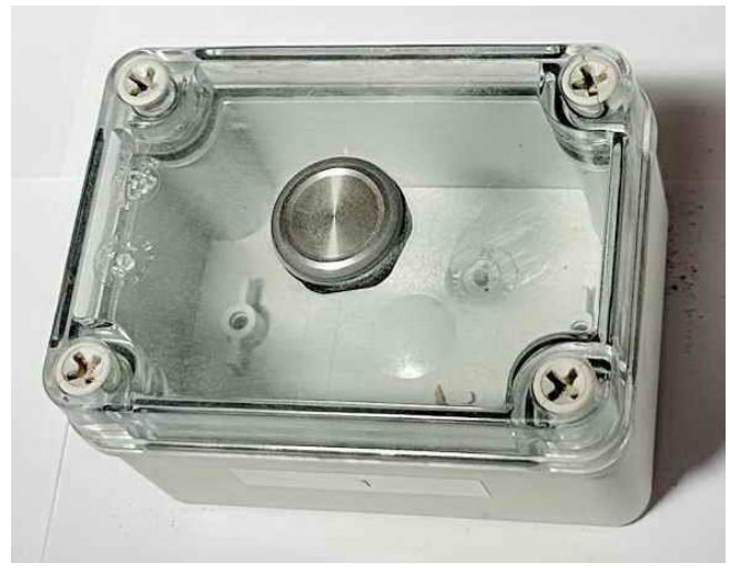
Fig. 15 Sample 1 after IP6KX, view 1.
