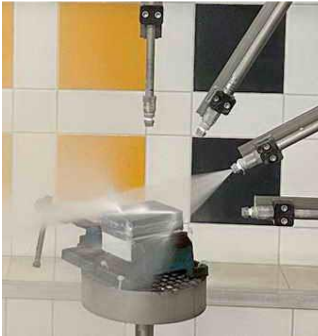
Fig. 12 DUT during spraying 30°, IPX9K.
