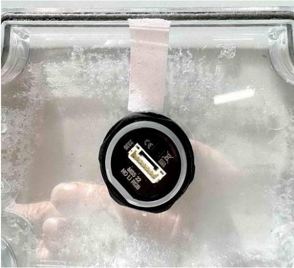
Fig. 20 Sample 1 dry test after IPX9K pos. 1.
