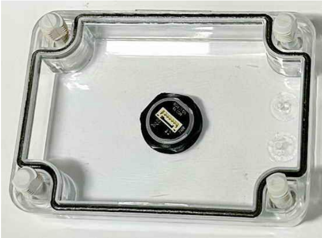
Fig. 34 Sample 3 after IP6KX, view 2.
