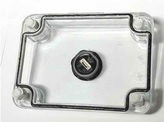
Fig. 16 Sample 1 after IP6KX, view 2.
