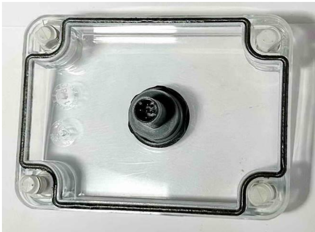
Fig. 25 Sample 2 after IP6KX, view 2.
