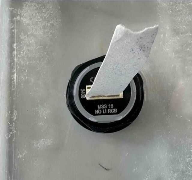
Fig. 49 Sample 4 dry test after IPX9K pos. 3.
