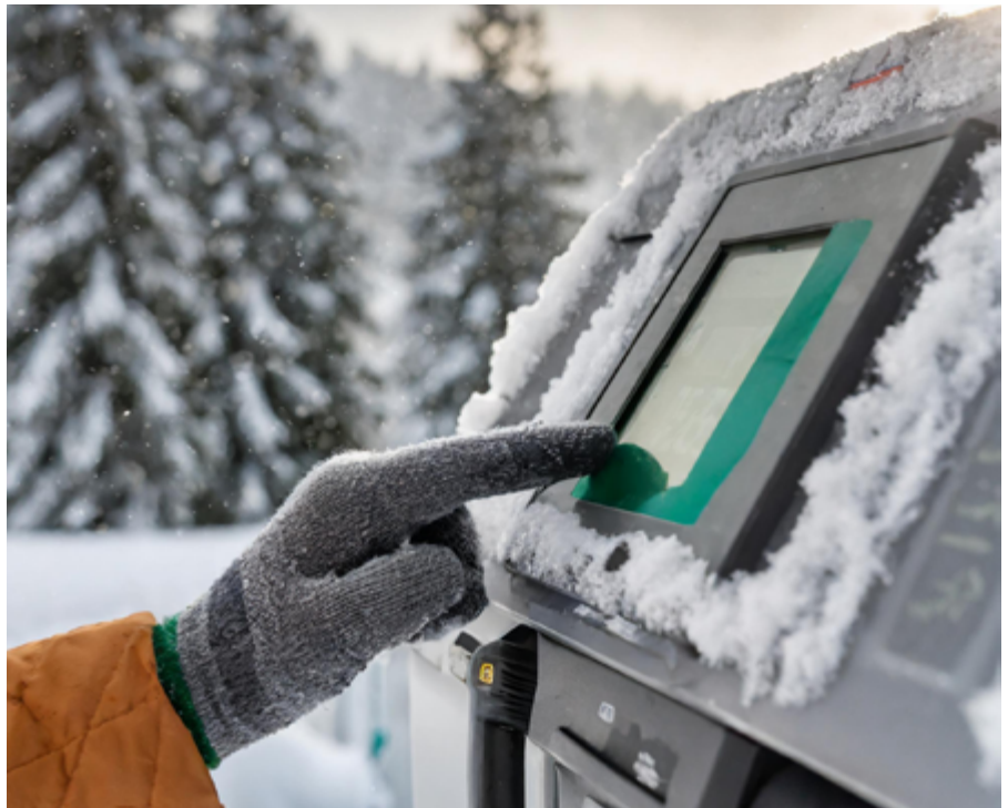
Outdoor applications require waterproof and sunlight-readable displays that are particularly robust and vandal-proof
